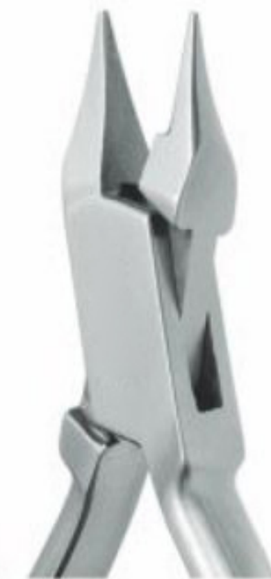
CSI-789 Slim Bird Beak Pliers Tapered Beak 12.5cm Max: .022"x0.25" (.56mm x .64mm) Wires
